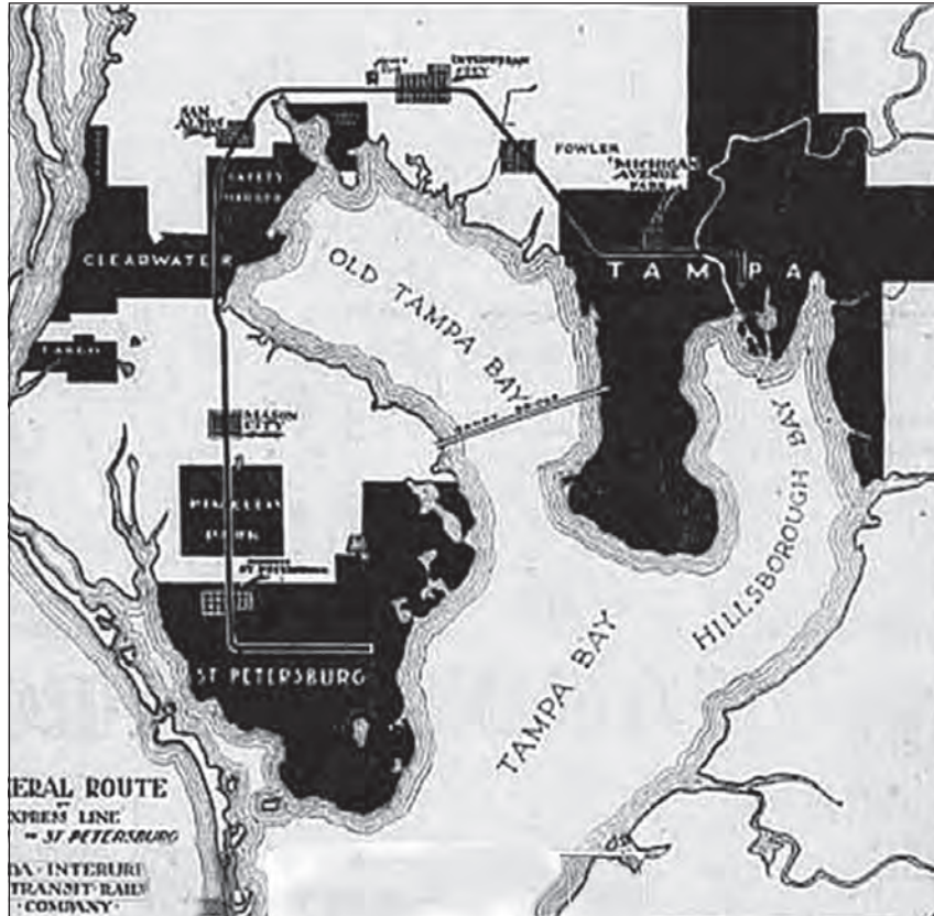
1925 proposed Interurban Rapid Transit route tying together Pinellas and Hillsborough counties. Most of the needed right-of-way was acquired, some grading undertaken, and a new bridge over the Hillsborough River partially built.
