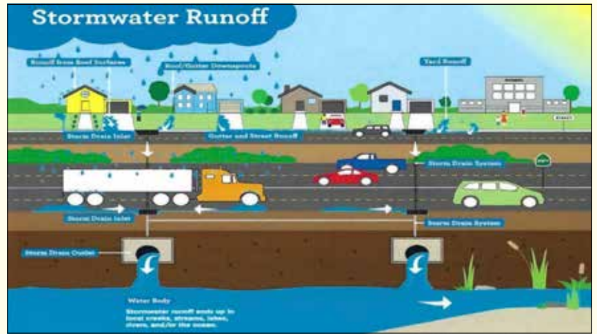
City image showing how the stormwater system works. Note the stormwater system is separate and independent from the wastewater system.
